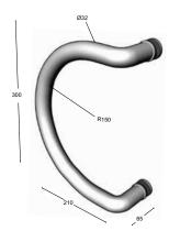
Circular pull handle for door thickness 10 - 70 mm.
