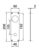
Back plate for ASSA Evolution and modular locks for lever handle and cylinder accessories.
