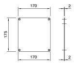
Square plate for doors where no lever handle and cylinder are required.
