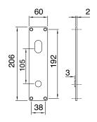
Back plate for ASSA Evolution and modular locks for cylinder and lever handle.
