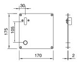
Square plate for ASSA Evolution and modular locks with cylinder and cylinder accessories.
