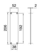
Back plate for internal doors, where no lever handle and cylinder are required.
